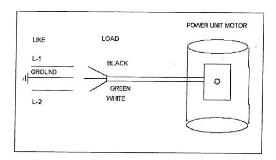
NOTE: All connections must be made by a Licensed Electrician in accordance with all State and Local Codes. Damage to motor caused by faulty wiring is not covered under warranty. Voltage required to operate—220 VAC single phase. For questions concerning electrical connections consult your distributor.
