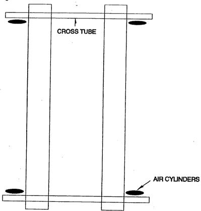
NOTE: It is helpful to rest the CROSS TUBES on the bottom lattices in the post prior to connecting chains.
