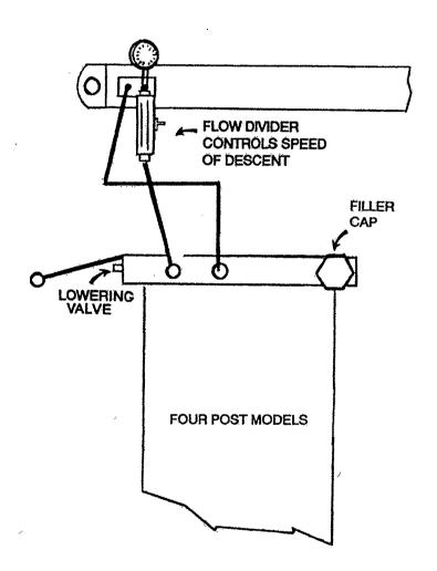
NOTE: It may be necessary to remove Allen plugs prior to installation of hose fittings.
